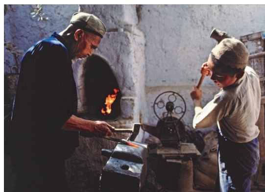
Uighur father and son team, near Kashgar, work together in forging a knife. The device next to the furnace is a blower for fanning the fires.
